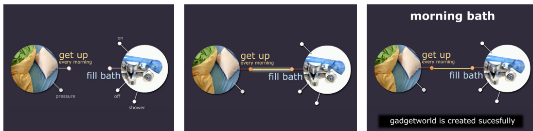
Figure 50: Handheld device: application creation (storyboard). The GUI corresponds directly to the connectivities – links (plug-synapse) model, using a simplified form of ‘line wiring’ connections, but suitable for ‘low-level’ applications.
