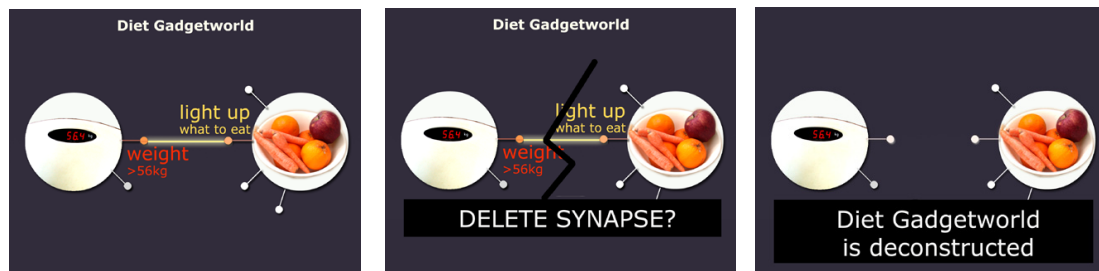
Figure 51: Handheld device (storyboard): deletion of a connection between artifacts, and therefore deletion of an application that has only one connection.
