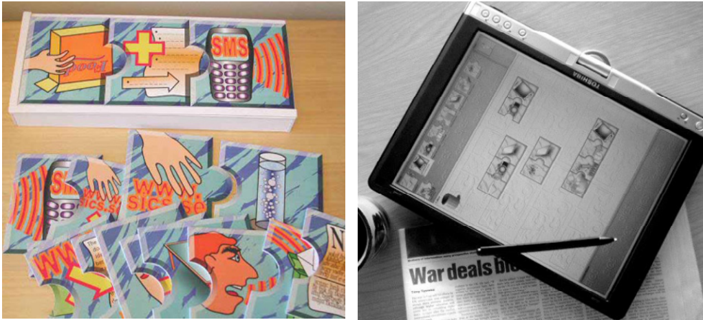
Figure 15: Left: the Paper Puzzle Editor using paper based identification technology. Right: the tablet editor and the editor screen. Each component is represented as a physical puzzle piece; a service is created by connecting pieces in a left-to-right order. (Source: ACCORD project website).
