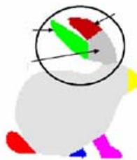
Figure 2.3.13. Segmentation of the ears of the bunny object. Three new components are generated and two of them are adjacent to only one part (taken from [KYL05])
