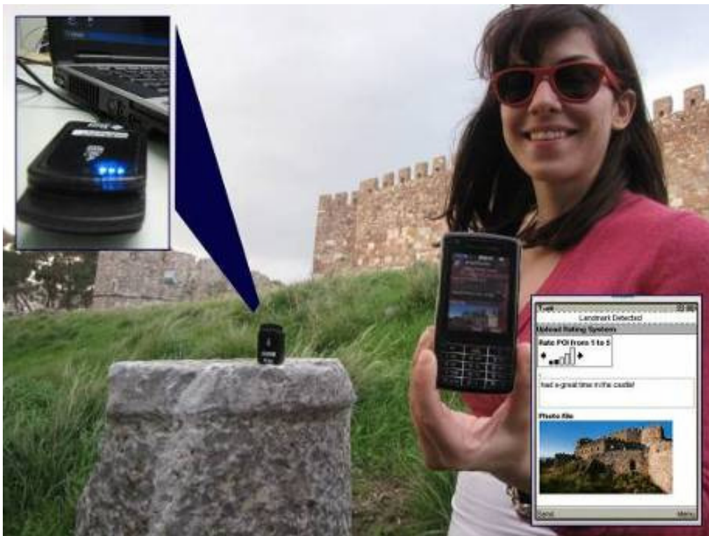
Figure 5-7. A user evaluator uploading content through a deployed WSN infrastructure (the SunSPOT node is shown on the top of the pillar, while the upper left part of the picture illustrates the sink which receives and forwards the tourist content to the remote web server).
