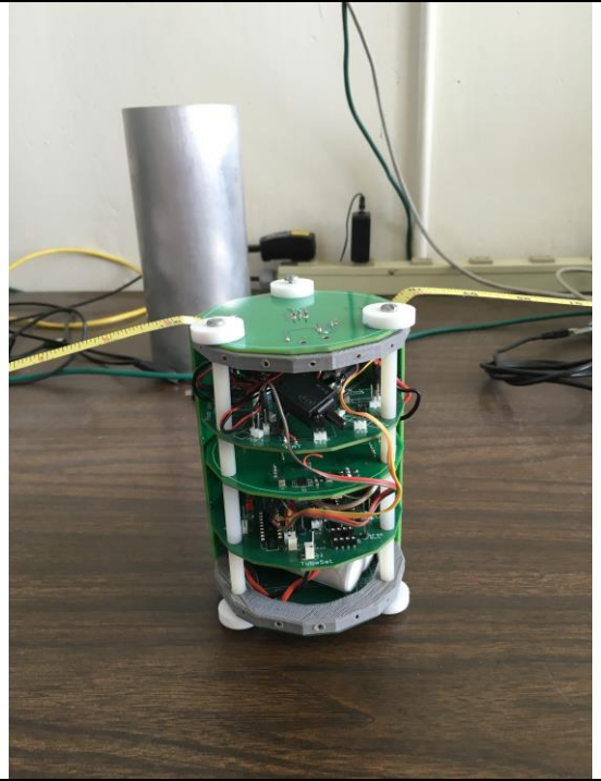
Side of Tubesat without solar panels showing all different connectivity through the boards
