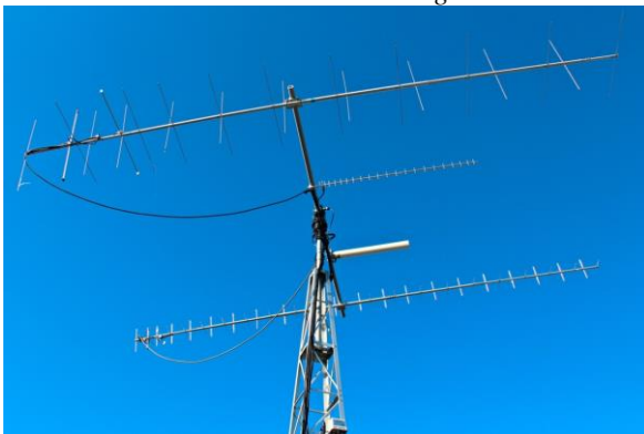
Old (right) and new (left) ground station antenna allocation. Newer antennas have extended receive profit for better microsatellite reception
