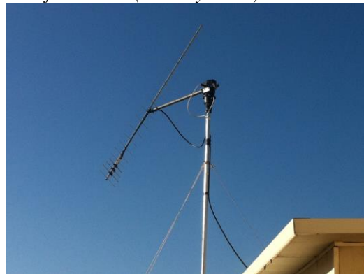
Old (right) and new (left) ground station antenna allocation. Newer antennas have extended receive profit for better microsatellite reception
