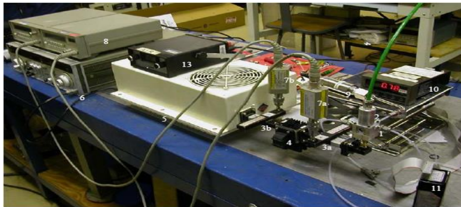
Figure 3. Experimental setup used for the 14.5-GHz MET testing (helium propellant supply tank and vacuum pump not shown).
