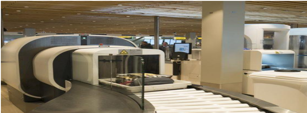
Figure 8: The new scans which analyze the interior of bags without need to take off metal or electrical objects.
