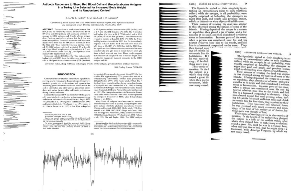
Figure 2-6: Projection profiles of a document (left) and the effect of skew (right) [19]
