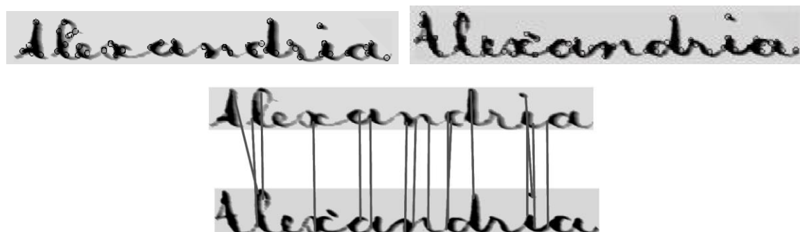
Figure 6-1: Harris corners (up) and recovered correspondences (down) [96]
