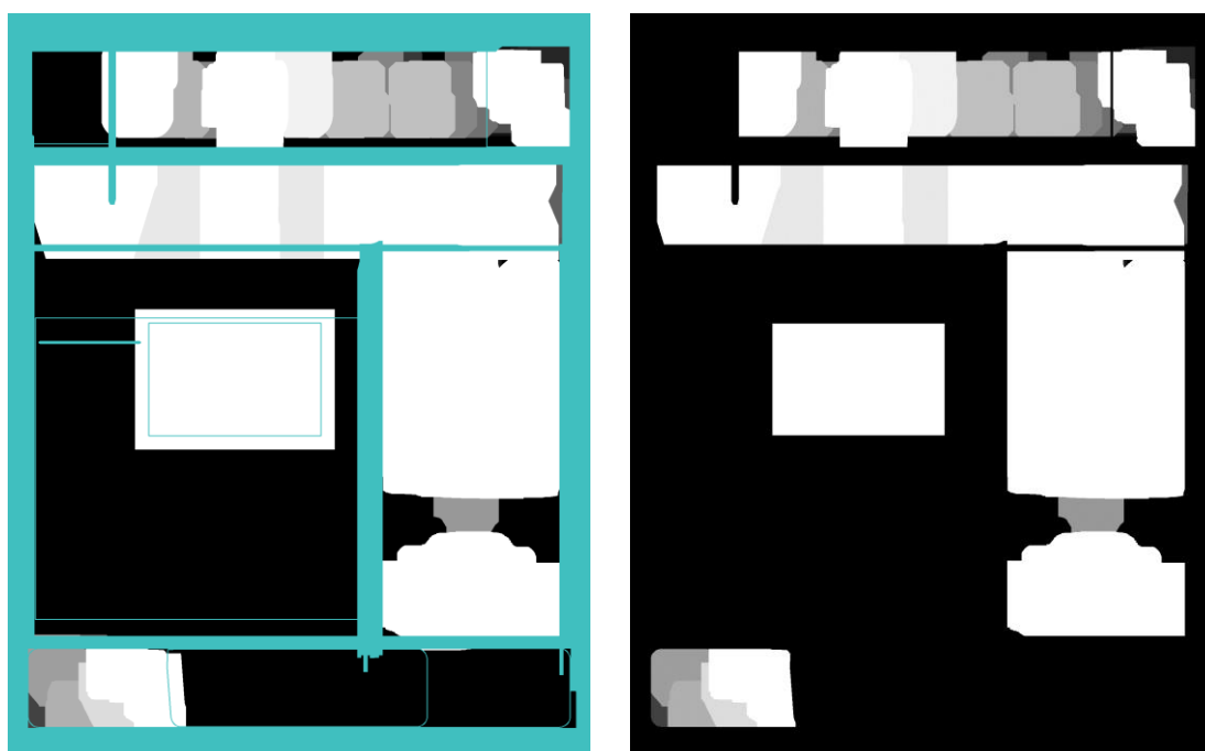
Figure 2-20. The dilated image of Figure 2.19 is ANDed with the invert separator mask
