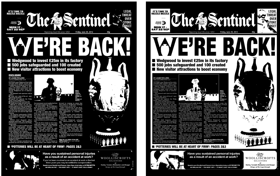
Figure 2-10: Binarization by the regional band (left) and Otsu's (right) thresholding
