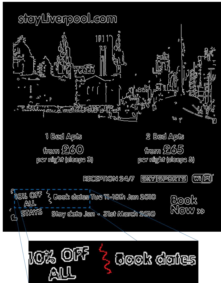
Figure 3-7: Example of a non-aligned component inside the outlined area
