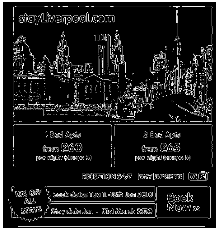
Figure 3-6: The result of Canny edge detection of the image in Figure 3.2
