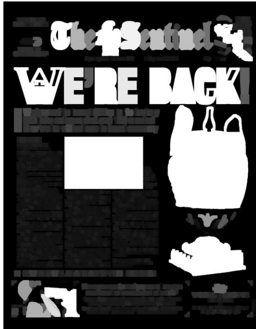
Figure 2-18: The image is dilated by an element of size one third of the x-height value
