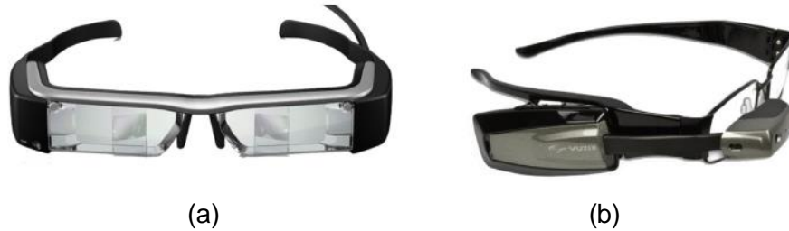
Figure 3.5 a) Binocular head-worn display, b) Monocular head-worn display, (Kim et al. , 2019)
