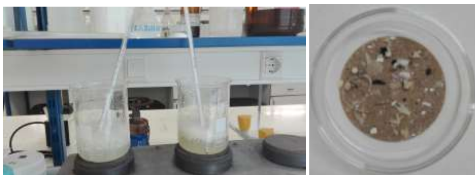
Figure 18. Wet digestion of samples with H 2 O 2 on a hotplate (left), dried sample after the filtration (right).
