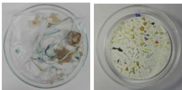
Figure 19. Large Microplastic sample- LMPs (left) and Small Microplastics sample-SMPs (right) analysing in stereo dissecting microscope.
