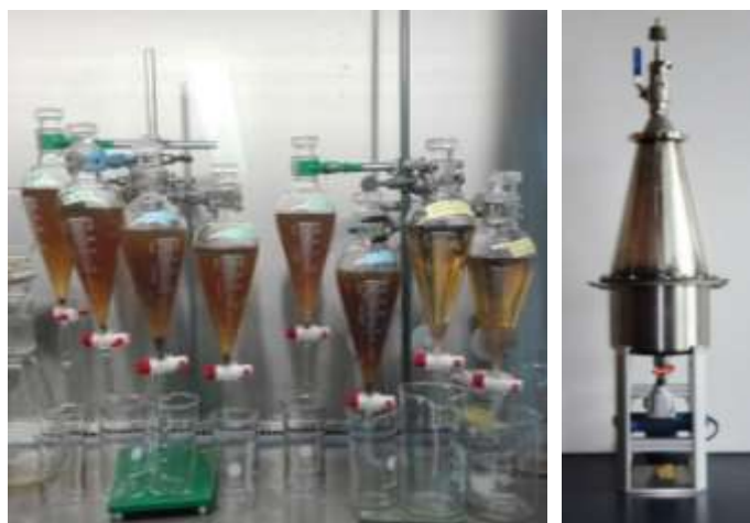
Figure 5. Microplastic separation methods; (i) density separation (Photo: Myrsini Lymperaki); (ii) MPSS separation (Photo: Imhof et al., 2012).
