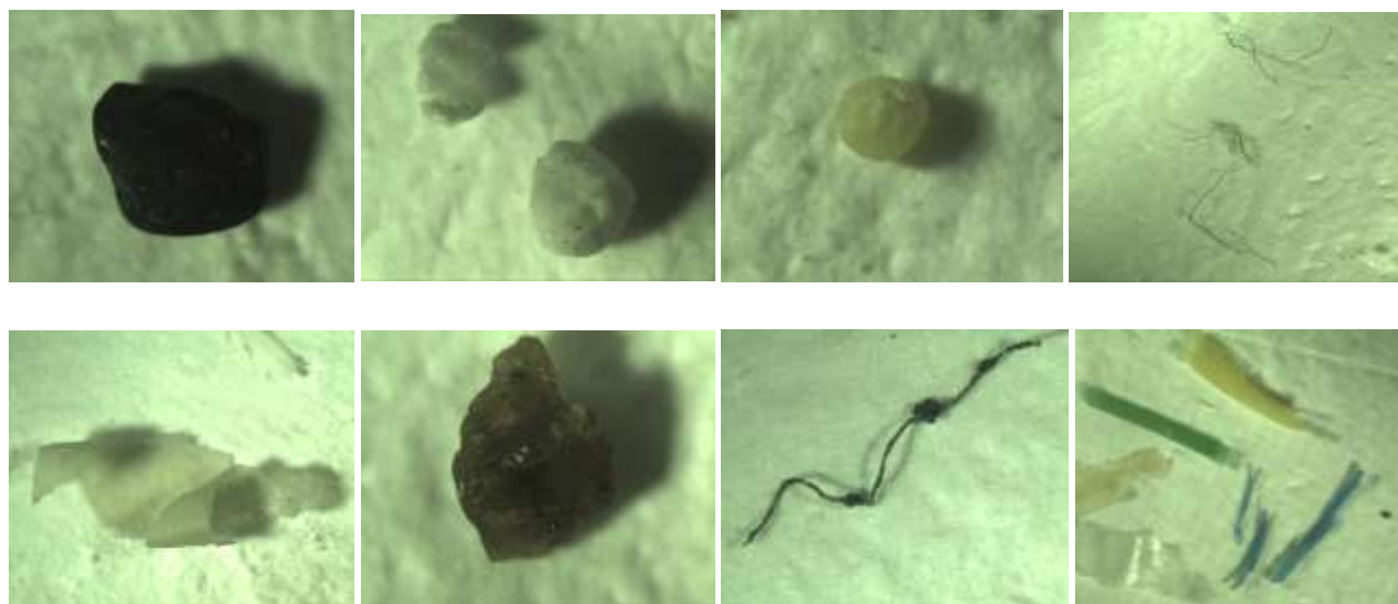
Figure 45. Different types of small microplastics; (i) fragment, (ii) foam, (iii) pellet, (iv) filaments, (v) fragment, (vi) fragment, (vii) filament, (viii) films.
