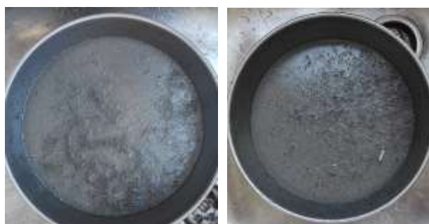
Figure 14. Small Microplastic samples-SMPs (300 \mu\text{m} -1mm) from different samplings in stainless steel sieves.
