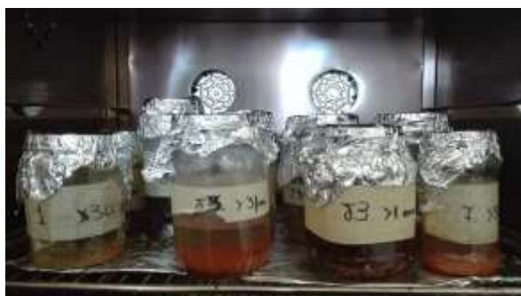
Figure 16. Sieved samples are dried in the oven to determine dry weight.
