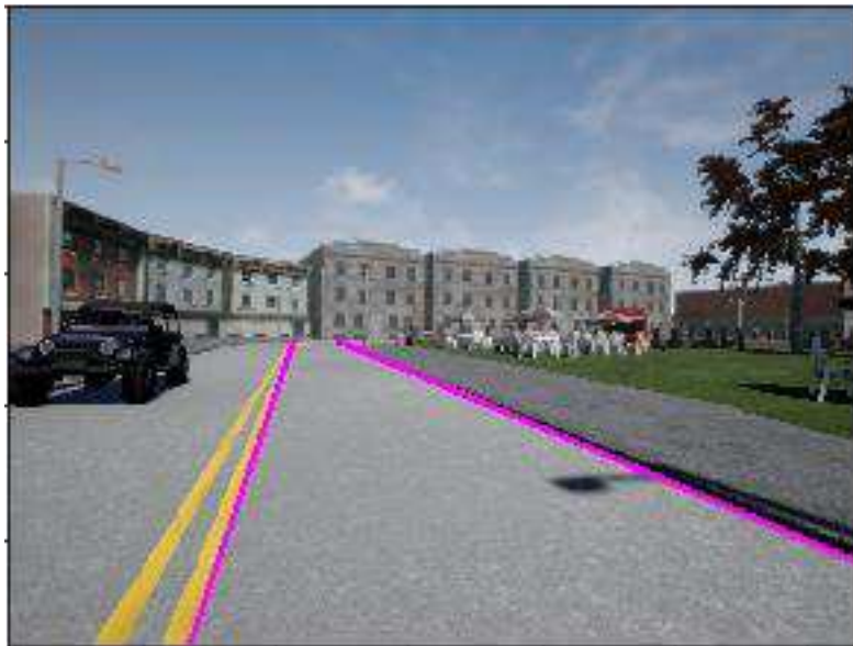
Figure 4.18 Lane estimation for the space where it is legally allowed for the autonomous vehicle to drive
