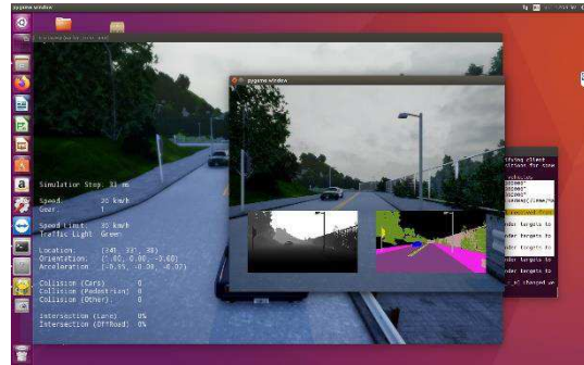
Figure 3.18 CARLA simulation environment with semantic segmentation and depth cameras (Screenshots from the DeOPSys Lab system)
