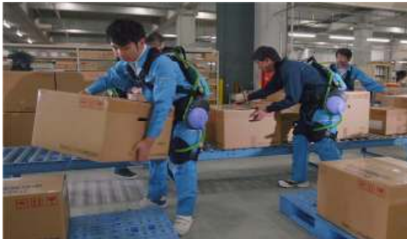
Figure 4.11 Based on electric power to function, exoskeleton support for workers aids them in day-to-day tasks or heavy and large item carrying. Such exoskeleton support is developed by Panasonic (Burgess, 2016).
