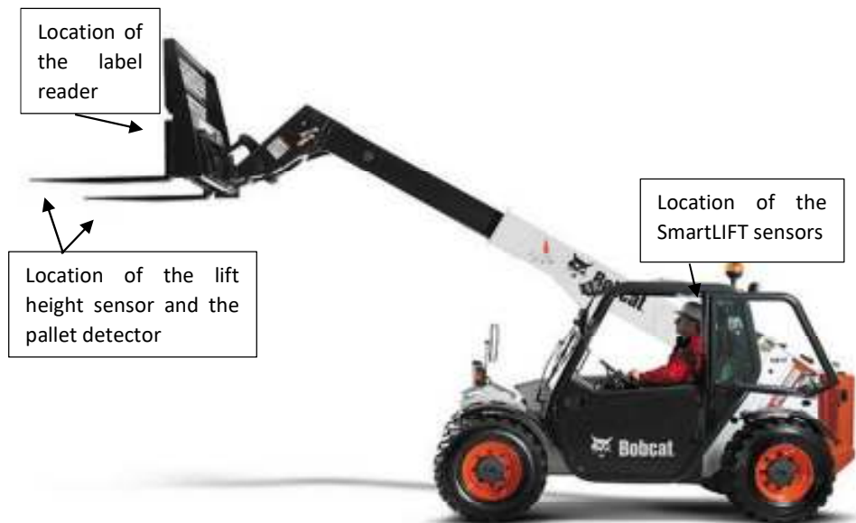
Figure 5.1 Showing the locations of the individual supporting technologies on a TELEHANDLER BOBCAT V417 (onestoprentalsales.com, 2018).
