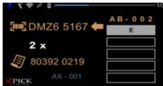
Figure 5.4 The information on the right concerns the aisle and the shelf for locating the item, while the information on the left concerns the item code, the quantity to be retrieved and the delivery note to be put on the box (Intel, 2015).
