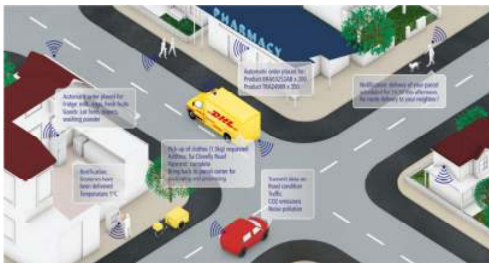
Figure 4.5 Shows how IoT redefines last-mile delivery. Features displayed: a) Automatic order placement, b) flexible address, c) delivery notification, d) returned goods request, e) collection route optimization (Macaulay et al., 2015).
