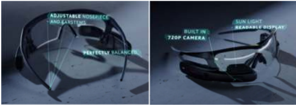
Figure 4.15 Displays the AR headset worn by workers and shows its features, such as the display and the camera (Intel, 2015).
