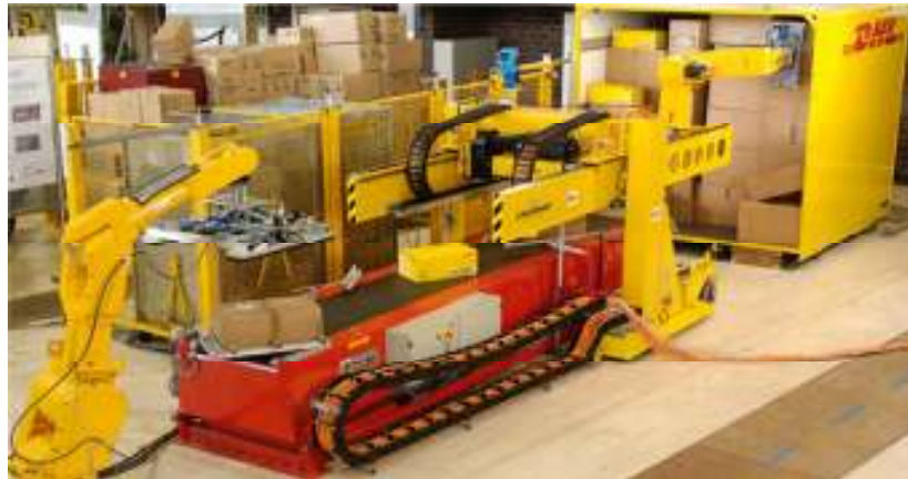
Figure 4.12 The DHL parcel Robot is a prototype developed by DHL and associates (Bonkenburg, 2016), which assists in unloading and loading of goods (I-scoop.eu, 2018).
