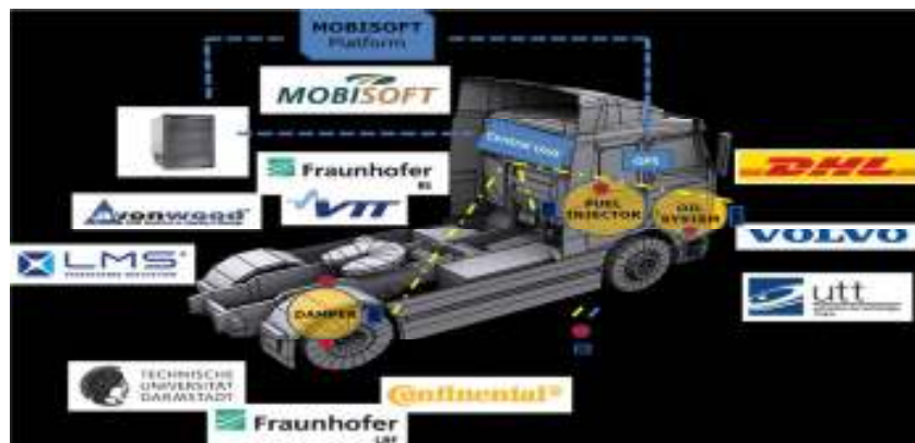
Figure 5.7 Many collaborating partners offered their expertise in developing the MODE project. As seen in this figure, the damper system, the fuel injector and the oil system have been embedded with sensors which send the data to the central system, which sequentially transmits them to a remote user (Avonwood, 2013).
