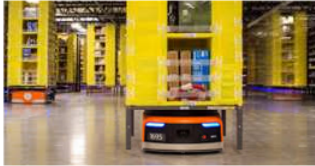
Figure 4.8 Goods to picker technology: Kiva moving a collection of items (Kim, 2015).
