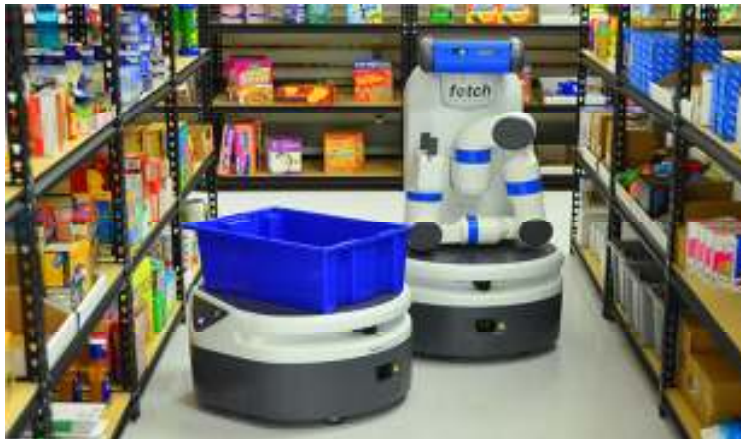
Figure 4.9 Fetch and Freight enabling full automation of the picking operation and offering a picker-to-goods solution (IEEE Spectrum, 2015).
