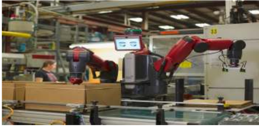
Figure 4.10 Baxter, designed by Rethink Robotics Company, assists in packing and sorting activities and tasks (Balinski, 2014).
