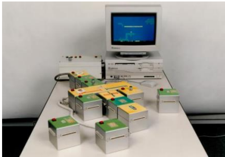
Figure 3-3: A collection of natural tangible programming blocks with electronic supplies using AlgoBlock (Suzuki & Kato, 1993)
