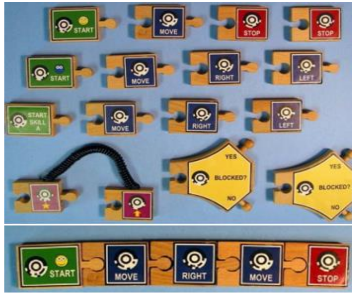
Figure 3-2: A collection of wooden tangible programming blocks using Tern (Horn et al., 2007)
