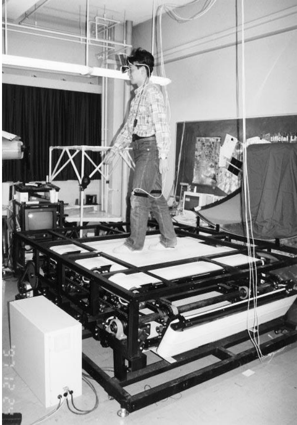
Figure 13. The Torus Treadmill device (Image credit: Path reproduction tests using a torus treadmill [149]).
