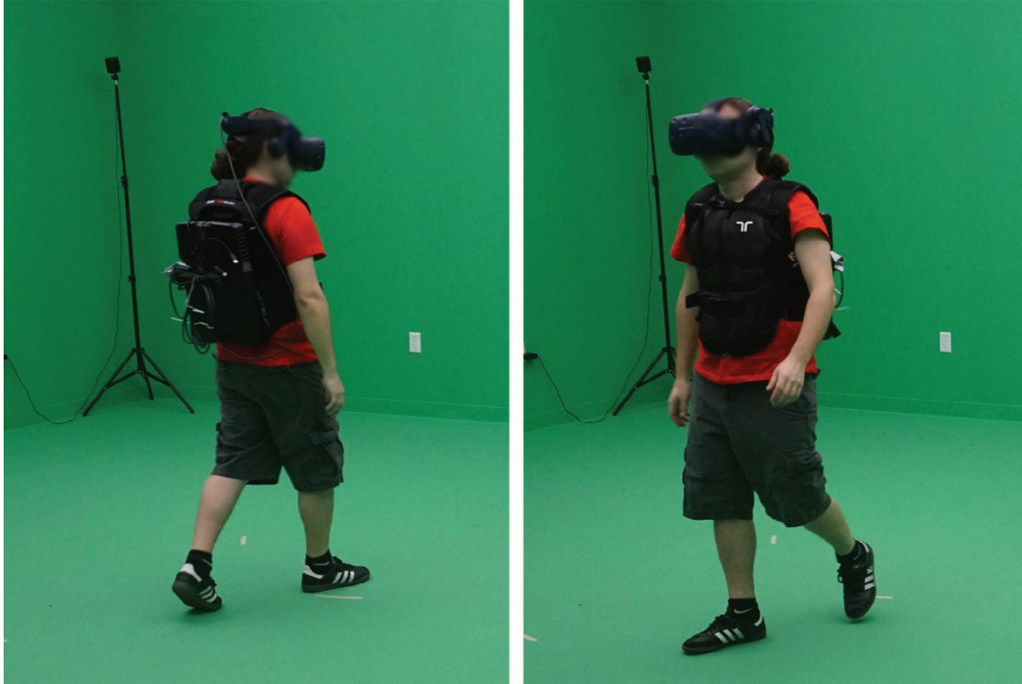
Figure 36. A participant wearing all devices (HTC Vive head-mounted display, bHaptics tactile vest, and MSI VR One backpack computer) used for study 3
