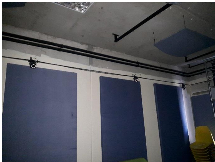
Figure 15: Bonita cameras placed around the ceiling of the motion capture room.
