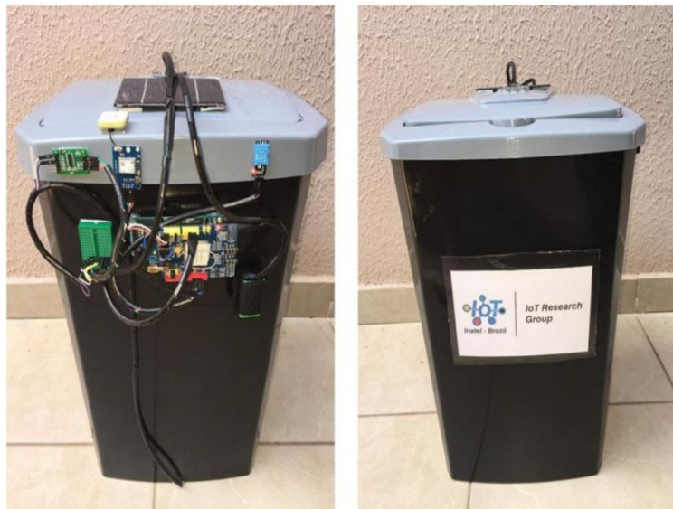
Figure 35 My Waste Bin, an IoT smart waste container, enabling real-time GPS tracking and weight monitoring
