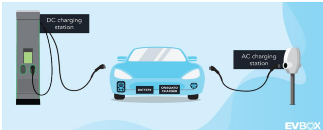
Figure 18: AC/DC charging, source: EVBOX
