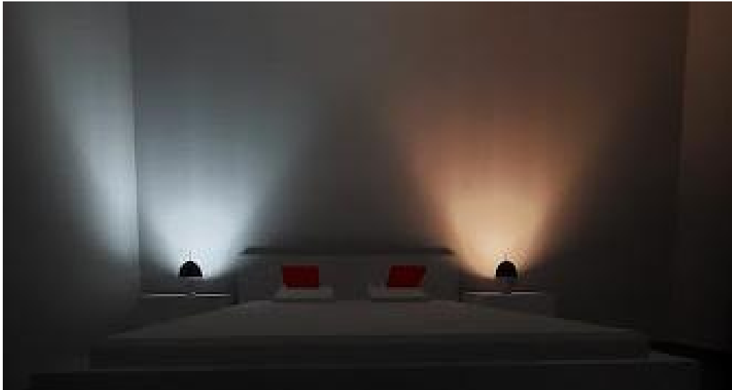
Image 25: Indicative photometric simulation in Dialux, different light color temperatures (left 3000K right 2200K)
